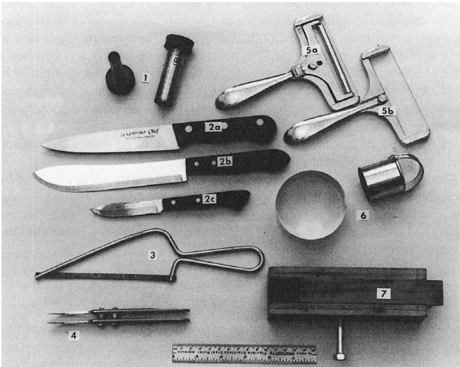
Figure 9.3 Some useful tools for shaping foods: 1, cork borers; 2, knives; 2a is the preferred type; 2b is undesirable because it is hollow ground and has a thick blade; 2c is undesirable because it is too small, is hollow ground and has a serrated edge; 3, small fine-tooth saw; 4, a pair of scalpels bolted together; 5a, household cheese cutter as purchased; 5b, cheese cutter with roller removed leaving space to cut samples up to 25 mm thick; 6, a large and a small cookie cutter; 7, a miter box with an adjustable slide.
