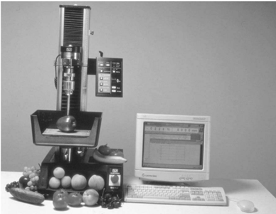
Figure 5.16 A model of the Instron often used on foods. (Courtesy of Instron Corporation.)
